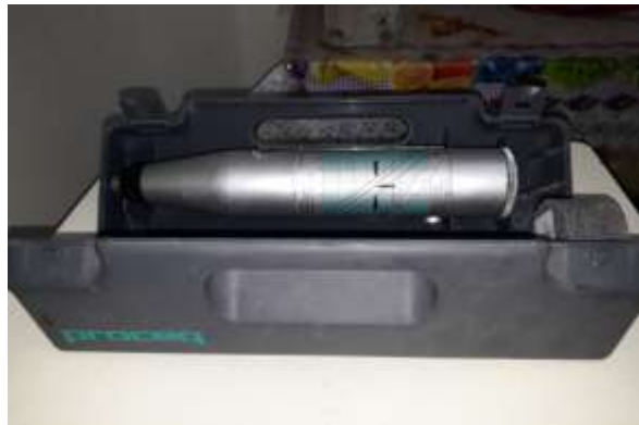
Fig. 1. Rebound Hammer Test
